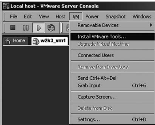
Figure 12.1 – Starting the VMware Tools installation
